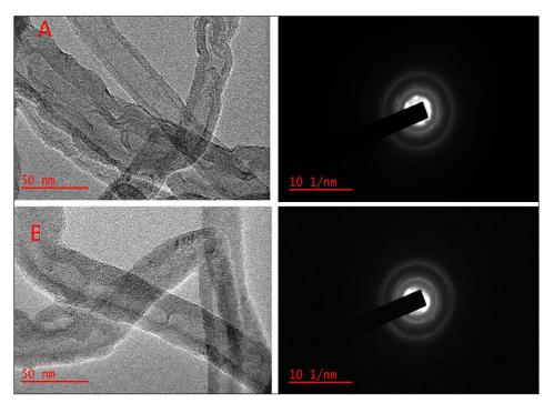
Fig. 9. TEM and SEAD of CNTs obtained from PP (A) and PE (B) over Fe-Co-Mo/CaCO<sub>3</sub> catalyst respectively
