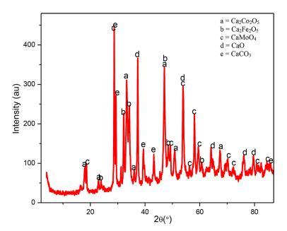
Fig. 1. XRD spectra of Fe-Co-Mo/CaCO<sub>3</sub> catalyst applied in the synthesize CNTs
