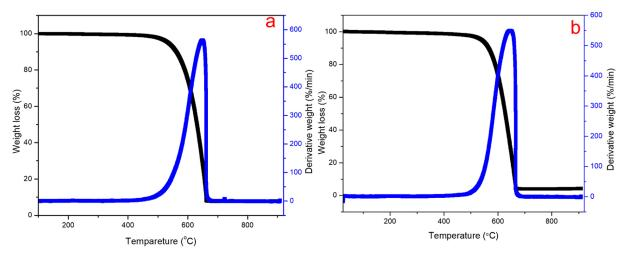
Fig. 8. TG/DTG profiles of as-synthesized CNTs from PP (a) and PE (b) as carbon sources over Fe-Co-Mo on calcium carbonate support
