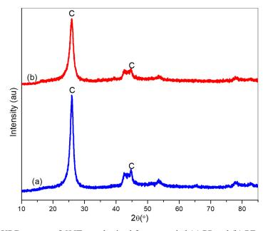
Fig. 4. XRD spectra of CNTs synthesized from recycled (a) PP and (b) PE as carbon sources over Fe-Co-Mo supported with CaCO<sub>3</sub> in a single CVD reactor system
