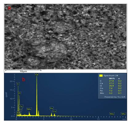
Fig. 2. (a) SEM morphology and (b) EDX spectra of Fe-Co-Mo/CaCO<sub>3</sub> catalyst
