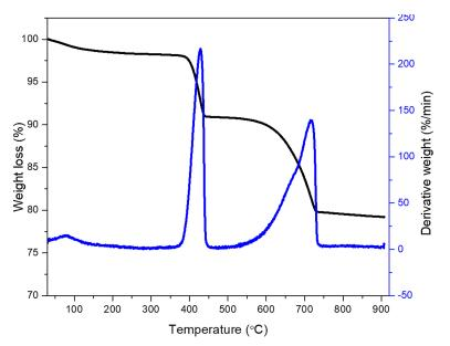
Fig. 3. TGA/DTG of prepared Fe-Co-Mo/CaCO<sub>3</sub> catalyst under air environment
