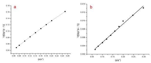
Fig. 7. BET-specific surface area plots of CNTs synthesized from recycled (a) PP and (b) PE over Fe-Co-Mo/CaCO<sub>3</sub> catalyst
