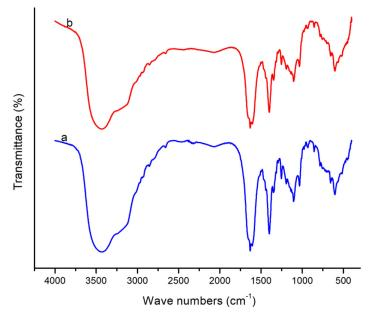
Fig. 5. FTIR spectrum of CNTs produced from recycled plastic wastes (a) PP and (b) PE over Fe-Co-Mo catalyst
