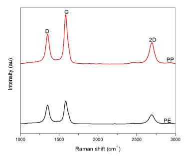
**Fig. 6.** Raman spectra of CNTs produced over a trimetallic catalyst of Fe-Co-Mo on CaCO<sub>3</sub> support using waste PP and PE as a carbon source in a single CVD reactor system
